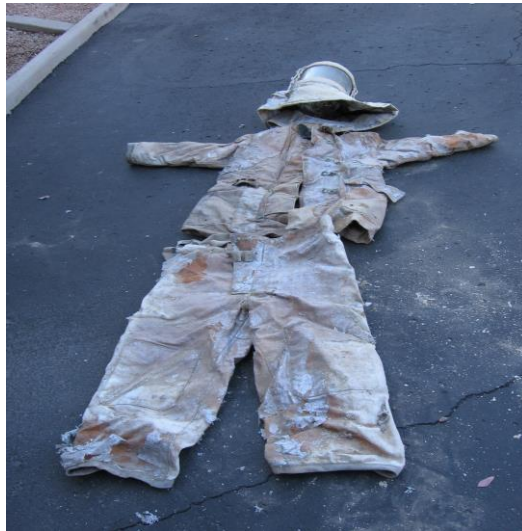
Used Protective Asbestos Clothing
